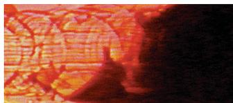
If the compression strength of the substrate is exceeded, portions of the substrate surface are crushed. This condition results in high energy noise bursts and normally increases the transverse force and effective friction.
