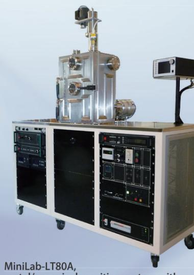
MiniLab-LT80A, metal/organic deposition system with, automated process control and extended rack
