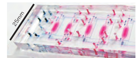
マイクロ回路デバイスの写真 Photo of body on a chip device. (fabricated by Dr. Hirai group of Kyoto University)
