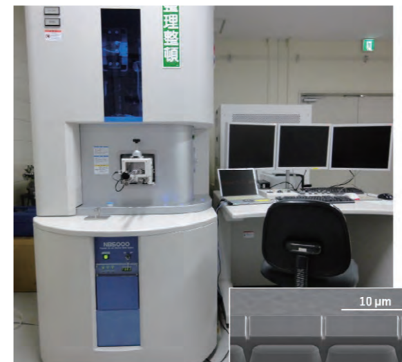
FIB-SEM装置および作製した流体デバイスの溝 FIB apparatus combined with SEM and fabricated channels in a fluidic device.
