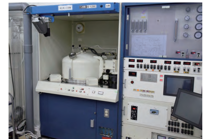
熱CVDによる低応力厚膜doped poly-Si Thermal CVD for low-stress, thick-film doped poly-Si
