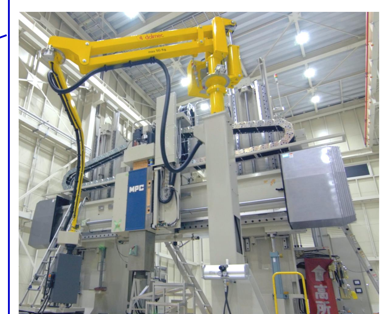
Large milling machine Height: 3.15m Stroke: 7.5m
